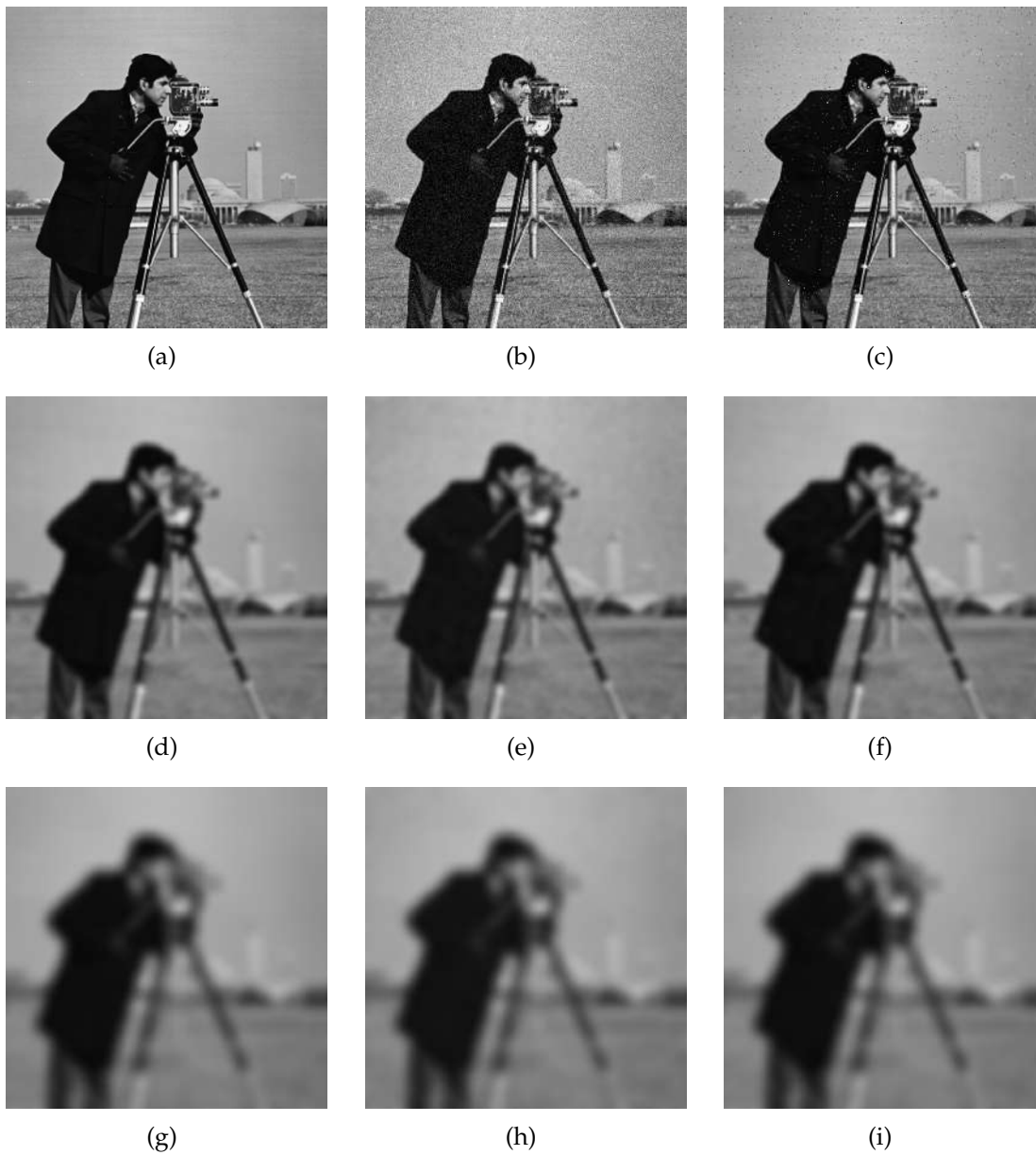
Figure 2.4: The original image and its linear diffusion filtered versions. a: Original Image, b: Gaussian Noise , c: salt and pepper. d,e and f: Image filtered by Linear-Filter after 5 Iteration. g,h and i: Image filtered by Linear-Filter after 20 Iteration
